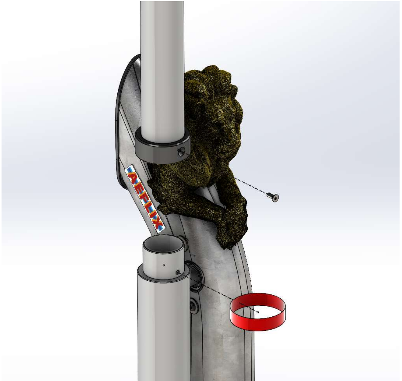
Figure 6. Installation of the beam
