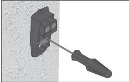
• If there is no signal, or if the signal is low, use the tuning screws to adjust the direction of the light to increase the signal.
